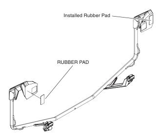
Install two Honda Pro-Connect<sup>™</sup> latches into the front carrier extender using a rubber spacer between each latch and the carrier extender. Secure the latches to the front carrier extender by installing a snap ring onto each latch from underneath the carrier extender.
