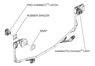
3. Lift the lever on each latch to unlock them. Place the front carrier extender onto the front carrier of the ATV. Line up each latch with its corresponding hole in the carrier then push each latch into its hole.
